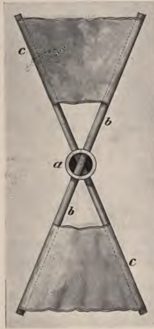
Fig. 16.—A fabric-covered screw with a very low efficiency.
